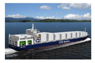
LNG is the cleanest fossil fuel available and significantly reduces carbon dioxide. These American built containerships are 720 feet long and 106 feet wide. They are the most advanced environmentally responsible vessels of their kind – reducing vessel sulfur emissions by 97 percent. The first ship, will enter service this year, the second ship is due in early 2016.
